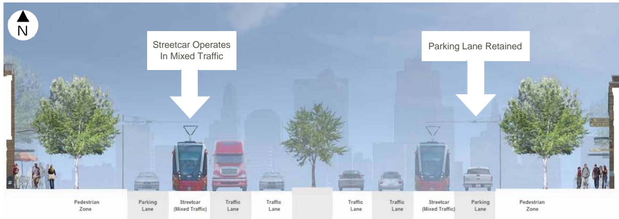
Figure 1-6: Mixed-Traffic Lane on Burlington
