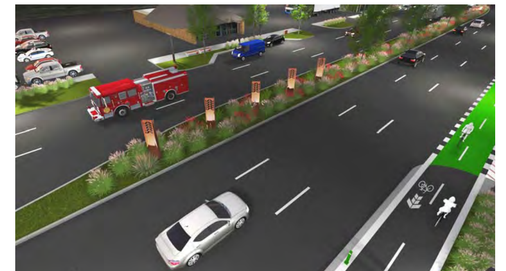
FIGURE 3.10 MEDIAN TREATMENT, MODEL VIEW
